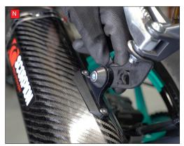
O & P) On the right side of the bike, remove the 2 bolts that hold the front/side plastic panel on.
