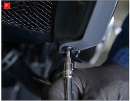
Y & Z) On the left side of the bike, remove the 2 bolts that hold the front plastic on.
