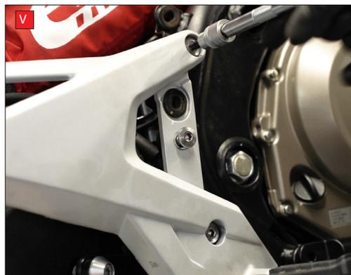
Q) Secure in place with the supplied washer and nut, don't fully tighten, you will do this in a later step.
