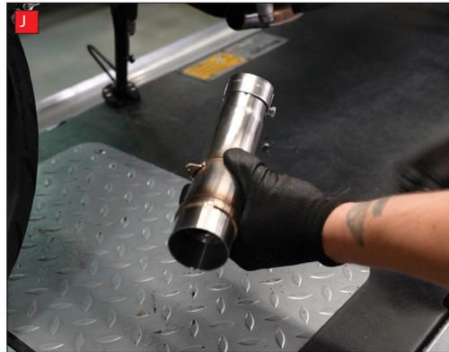
I) Remove the unused sleeve and rubber mount from the left side of the bike. This is not used when installing the Scorpion Slip-on Exhaust.
