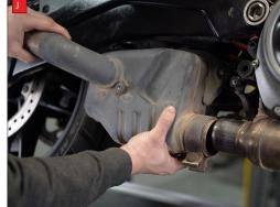
I) Remove the centre silencer mounting bolt.
