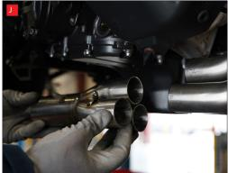
I) Starting from the left loosely fit the scorpion header pipes. Do not fully tighten until the whole system is fitted.
