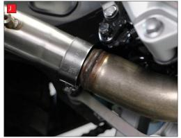
I) Attach the springs between the silencer and the connecting pipe.
