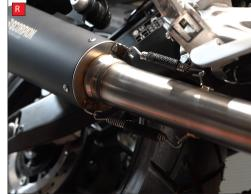
Q) Fully tighten the rear silencer mounting hardware.
