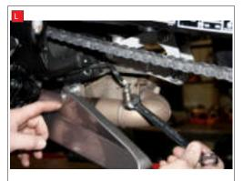
L) Put the Lambda sensor into the CP668, if no lambda sensor is on bike then leave in blanking plug, make sure the Lambda or blanking plug is tight.
