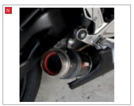
O) Fully tighten the clamp on CP668 to O.E system.
