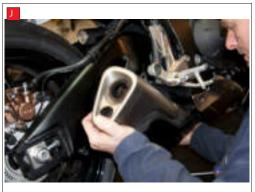
I) Remove O.E silencer mounting bolt, keep this bolt as it will be needed later on in fitting Scorpion Exhaust.
