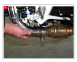
J) Introduce the Scorpion connecting pipe CP 436 to the header pipe with the clamp on the CP 436.
