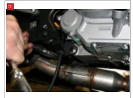
E) Attach Scorpion Header Pipe, using the O.E nuts, and making sure you reconnect the breather pipe, making sure the O.E retainer spring is on the pipe.
