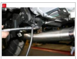
I) Bolt the Scorpion silencer to the O.E mounting bracket and fully tighten. Then fully tighten the bolt that gose onto the Scorpion silencer mounting bracket.
